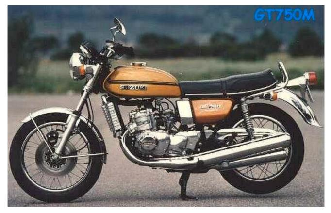
Major performance related changes raised claimed hp from 67 to 70. gearing was raised to p[ass noise emission test and the new changes led to a loss of bottom end but a slight improvement at the top. All new exhaust and crossovers are eliminated. Exhaust port raised, intake port lowered, 0.2mm off head to raise compression to 6.9:1 Forks changed to eliminate chrome top dust seal cover. Fork springs retained by circlip and fork internals also changed.
